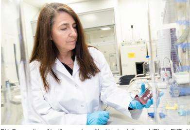
BU: Preparation of textile samples with skin simulating gel (Photo FKTe.V.)
